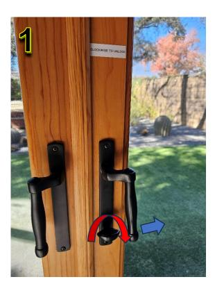
2. You will hear a strong \*click\* when you use the handle to open the door. This means the latch is secured in the "**open**" position.
